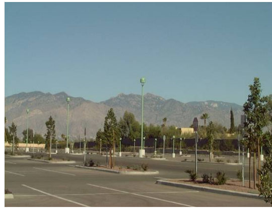
Figure 3 - Every Other Row Option Parking Lot with Fully Shielded Luminaires ( Monrad Engineering, Inc. )
