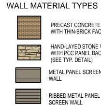
PRECAST CONCRETE WITH THIN-BRICK FACE HAND-LAYED STONE VENEER WITH PCC PANEL BACK-UP (SEE TYP. DETAIL) METAL PANEL SCREEN WALL RIBBED METAL PANEL SCREEN WALL
