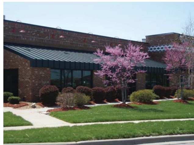
The eave provides shade for the windows and helps break up the horizontal massing
