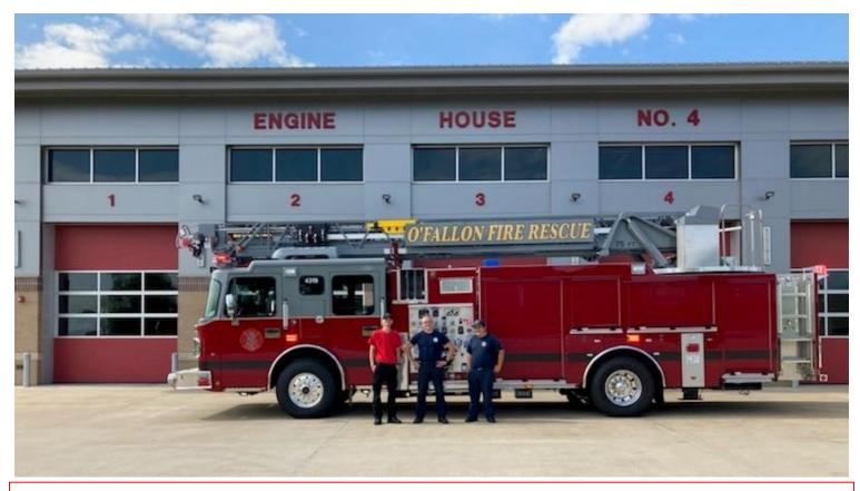
O'Fallon Fire Rescue's newest truck, a 2022 Spartan 75' Quint, was purchased as part of our established vehicle replacement schedule. Typically, we keep ladder trucks 20 years and fire engines 15 years. In this case, we originally ran this truck for both ladder and engine operations. Hence, it's replacement at the 15-year mark. The new truck will be run as a traditional ladder with plans to keep it the full 20 years. The new truck will be housed at Engine House #1 on E Washington St.
